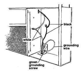
Connect the white and black wires of the power supply cable to the white and black leads in the hood with twist-on connectors.
